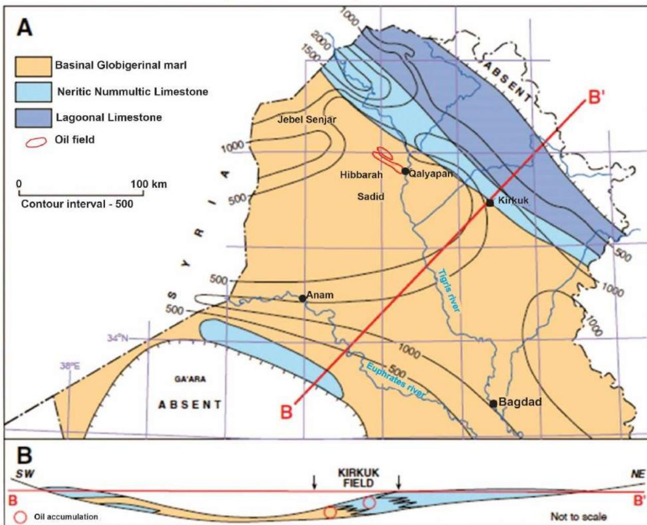
**Fig. 12.** (A) Isopach and paleogeography map of the Middle-Upper Eocene section of northern Iraq. This interval constitutes the lower Main Limestone reservoir at the Kirkuk Field. (B) Schematic cross-section across the basin in Eocene times showing the carbonate platform that fringed the NW-trending interior seaway or intra-shelf basin with the relative location of Kirkuk marked (Dunnington, 1958). Line of section is shown in (A)
