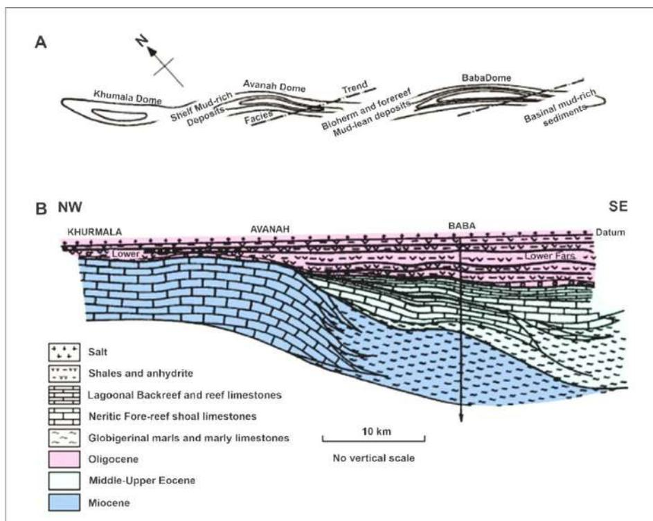
**Fig. 9.** Stratigraphy and depositional environments of Tertiary strata in the Kirkuk Field (Majid and Veizer, 1986). Main Limestone reservoir layers (which are shown in the cross-section in Fig. 8) and thickness are also given (Al-Naqib et al., 1971)
