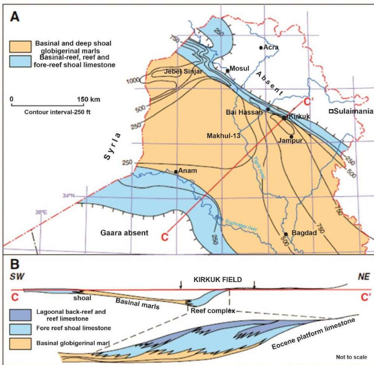
**Fig. 13.** (A) Isopach and paleogeography map for the Oligocene section of northern Iraq. This interval constitutes the Upper Main Limestone reservoir at the Kirkuk Field. (B) Schematic cross-section across the basin in Oligocene times. The detailed inset shows how several cycles of reef development prograde basin wards from below the level of the Eocene platform edge (Dunnington, 1958). The relative location of Kirkuk is marked. Line of section is shown in (A)
