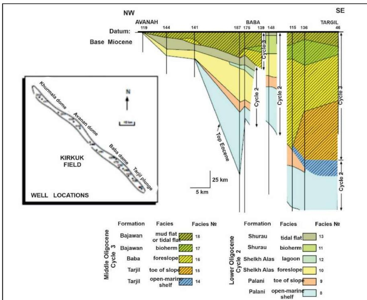
**Fig. 11.** NW-SE schematic stratigraphic cross-section through the Kirkuk Field showing lateral variation in relative thickness and facies of the Oligocene interval (Majid and Veizer, 1986). Inset map gives well locations
