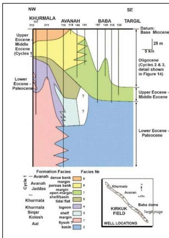
**Fig. 10.** NW-SE schematic stratigraphic cross-section through the Kirkuk Field showing lateral variation in relative thickness and facies of the Upper Paleocene-Upper Eocene interval (Majid and Veizer, 1986)
