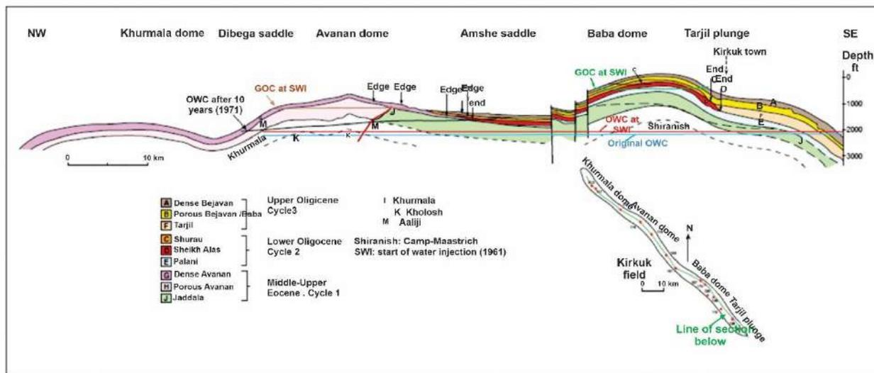
**Fig. 6.** NW-SE structural cross-section through the Kirkuk Field showing reservoir geometry and fluid contacts (Alamir, 1972). The main reservoir unit over the Khurmala and Avanan domes does not reach the Baba dome, while reservoir units of the Baba dome and Amshe saddle are younger and thin rapidly onto the Avanan dome (See Fig. 10 for explanation of lithostratigraphic units and depositional facies)
