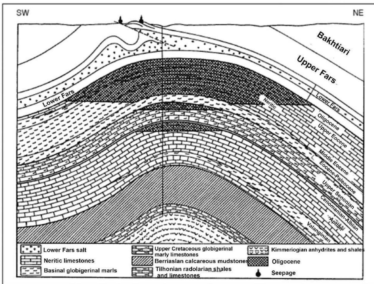
**Fig. 7.** SW-NE schematic structural cross-section of the Kirkuk structure showing three main oil accumulations (Dunnington, 1958)
