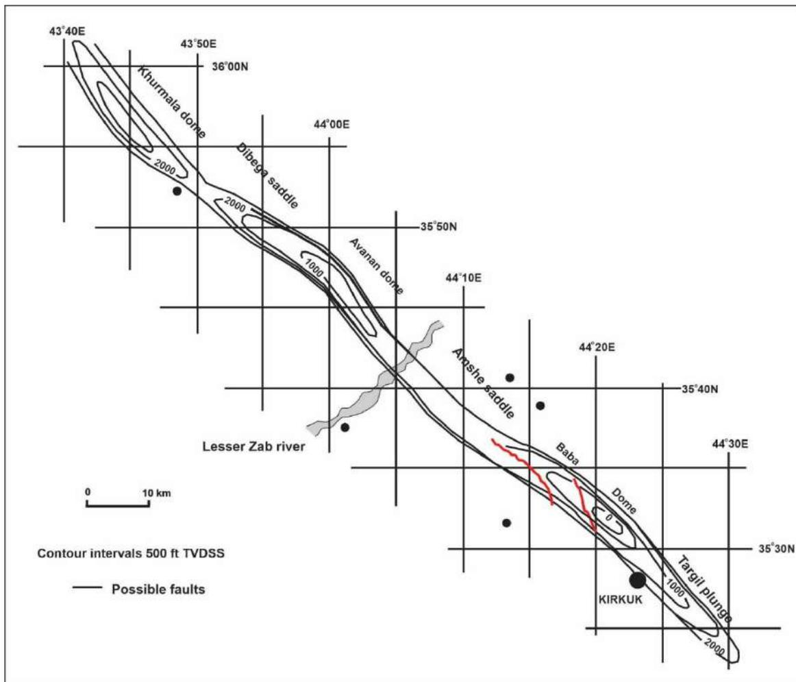
Fig. 2. Depth structure map on the near Top Main Limestone reservoir (modified after Sims and Shafiq, 1960)
